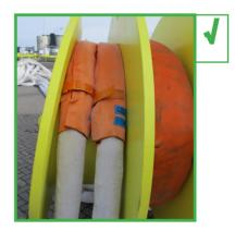
The D:d ratio and the bending radius between the sling and lifting gear/shackle must be considered. Extreema® slings under 150T should have a minimum of D:d ratio 1:1; everything above 150T is 1,5:1. If the WLL exceeds 300T or you require specific information consult the datasheets on our website: extreemasoftslings.com or contact the manufacturer or a dealer.
